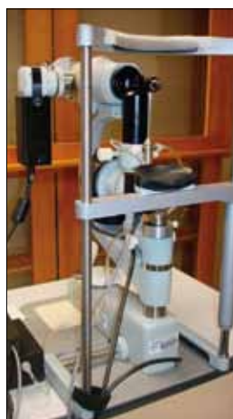
Figure 1. Computerized episcleral venomanometer for automated, objective, noninvasive measurement of episcleral venous pressure.
