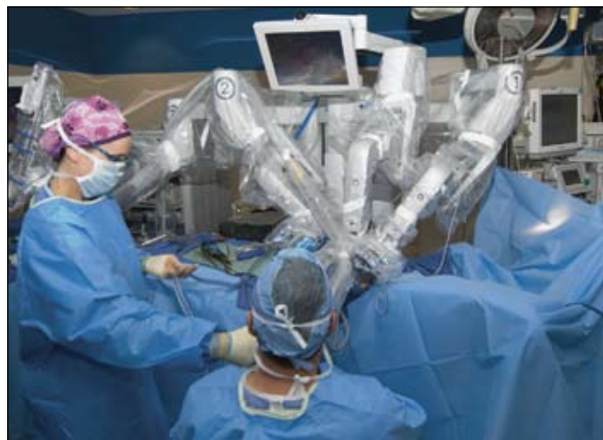
Figure 2. The surgical robot working platform with articulated arms that are in contact with the patient.
