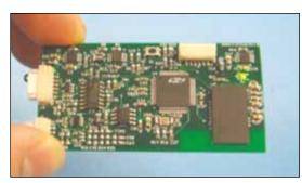
**Figure 1.** *Circuit board of the Wireless Instantaneous Neurotransmitter Concentration Sensing System device. The device is able to wirelessly detect neurotransmitter level changes in the brain.*
