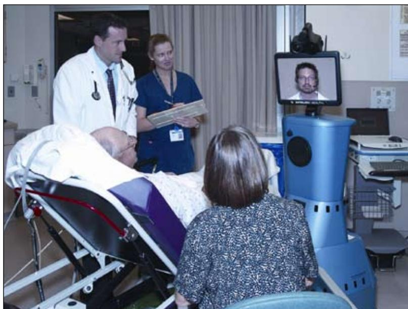
**Figure 1.** Dr Bart Demaerschalk operates a remotely controlled robot telemedicine platform, which allows him to assess and treat a patient with acute stroke in a rural hospital in an underserved community hundreds of miles away.
