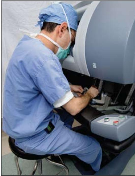
**Figure 1.** *The surgeon workstation of the surgical robot.*
