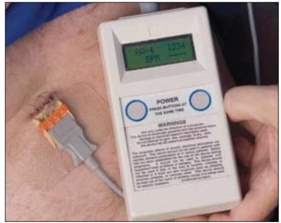
**Figure.** An external electronic stimulator is attached via wires through the skin to 4 electrodes implanted in the diaphragm near the phrenic nerves. The device generates an electric impulse that triggers the diaphragm to contract and allows air to fill the upper and lower parts of the lungs.
