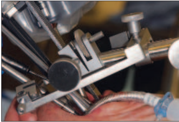
Figure 2. The surgical robotics system offers improved access to the oral cavity and better maneuverability.
