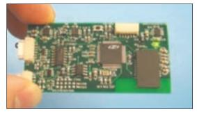
**Figure 1.** *Circuit board of the Wireless Instantaneous Neurotransmitter Concentration Sensing System device. The device is able to wirelessly detect neurotransmitter level changes in the brain.*
