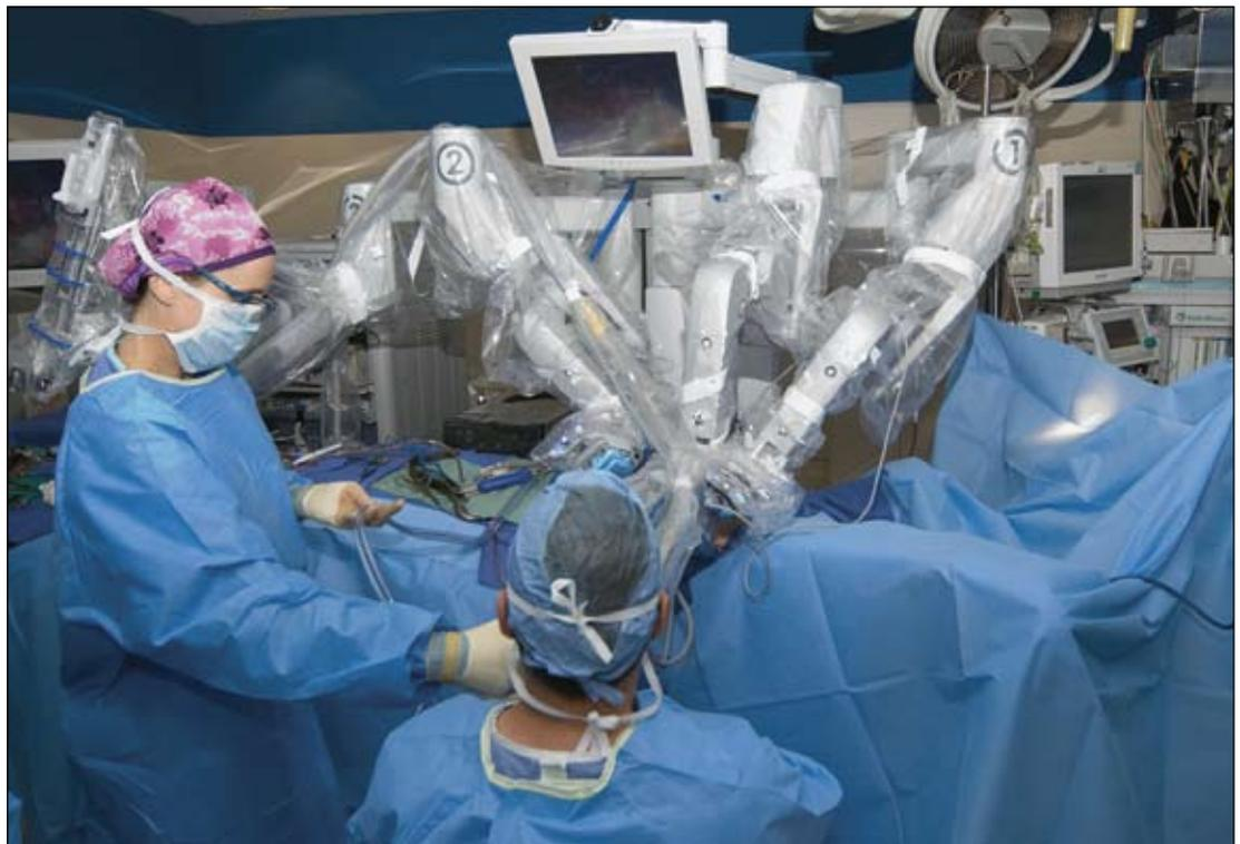
**Figure 2.** *The surgical robot working platform with articulated arms that are in contact with the patient.*
